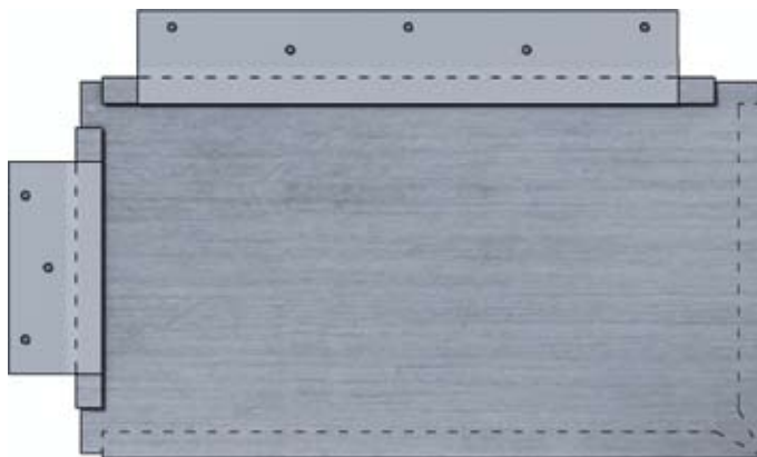
Continuous cleats are used in edges and corners to accommodate potential high wind suction loads.
