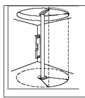
A plate is fixed to the floor then a column is attached to the plate. All the other parts including the treads are slid over the column and then topped off with the landing which is attached to the upper floor.
