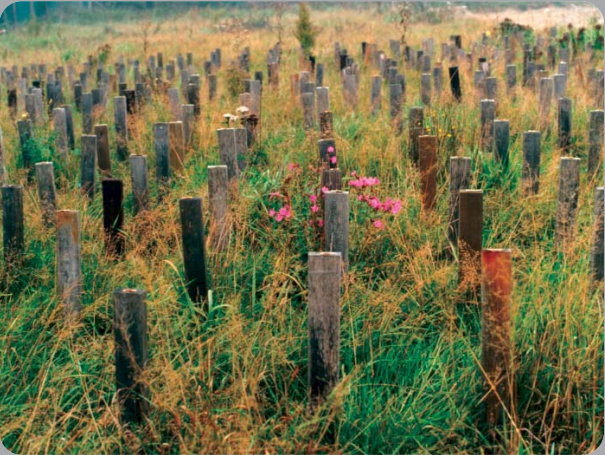
The picture above shows extensive “graveyard” field trials over a 16 year period which demonstrates Accoya® Class 1 durability rating which exceeds some of the worlds most durable timber species, including Teak.
