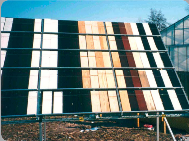
The picture above shows extensive field trials over a 10 year period that prove Accoya® has excellent coatings compatibility. The field testing has been undertaken for 10 years on south facing stands at 45° angles to demonstrate that Accoya® can offer market leader paint warranties in the most severe elevations.
