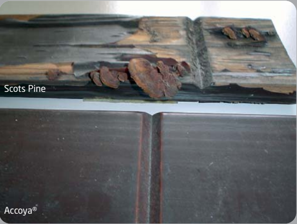
The picture above shows a 10 year outdoor field test of Scots Pine and Accoya® with a translucent coating. The picture demonstrates that Accoya® is durable, rot and UV resistant, easily maintained and has exceptional coatings performance.
